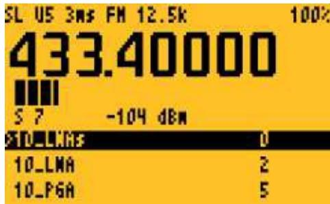
When you press the transmit button, you will enter VFO mode with a fixation on the selected frequency or channel (if you have saved this frequency with the 2 button). By holding the 2 button in home screen mode, you can add a channel to the scan list (s1-s5).
